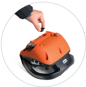
External removable EEPROM SIM module
